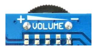
\*As a general rule for instruments and audio systems, always perform all wiring and connection of cables before powering-on the equipment, it is recommended to power-on the smartWAV2 + MIDI Adapter board while the volume potentiometer it's at the lowest volume position, then adjust the volume.
