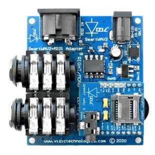
The SmartWAV 2 is an Intellectual Property smart high-end audio processor, when mounted on the MIDI Adapter board, it is called the SmartWAV2 + MIDI Adapter and the processor always operates in "MIDI Mode".
