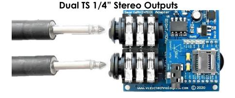
\*Never mix connection types or use both TS and TRS cables, use only one type of wiring and follow always the above connections.
