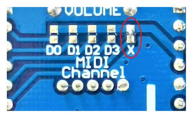
When a jumper pad is soldered: it is connected to VCC or closed, when the pad is left unsoldered: it is connected to GND or open.
