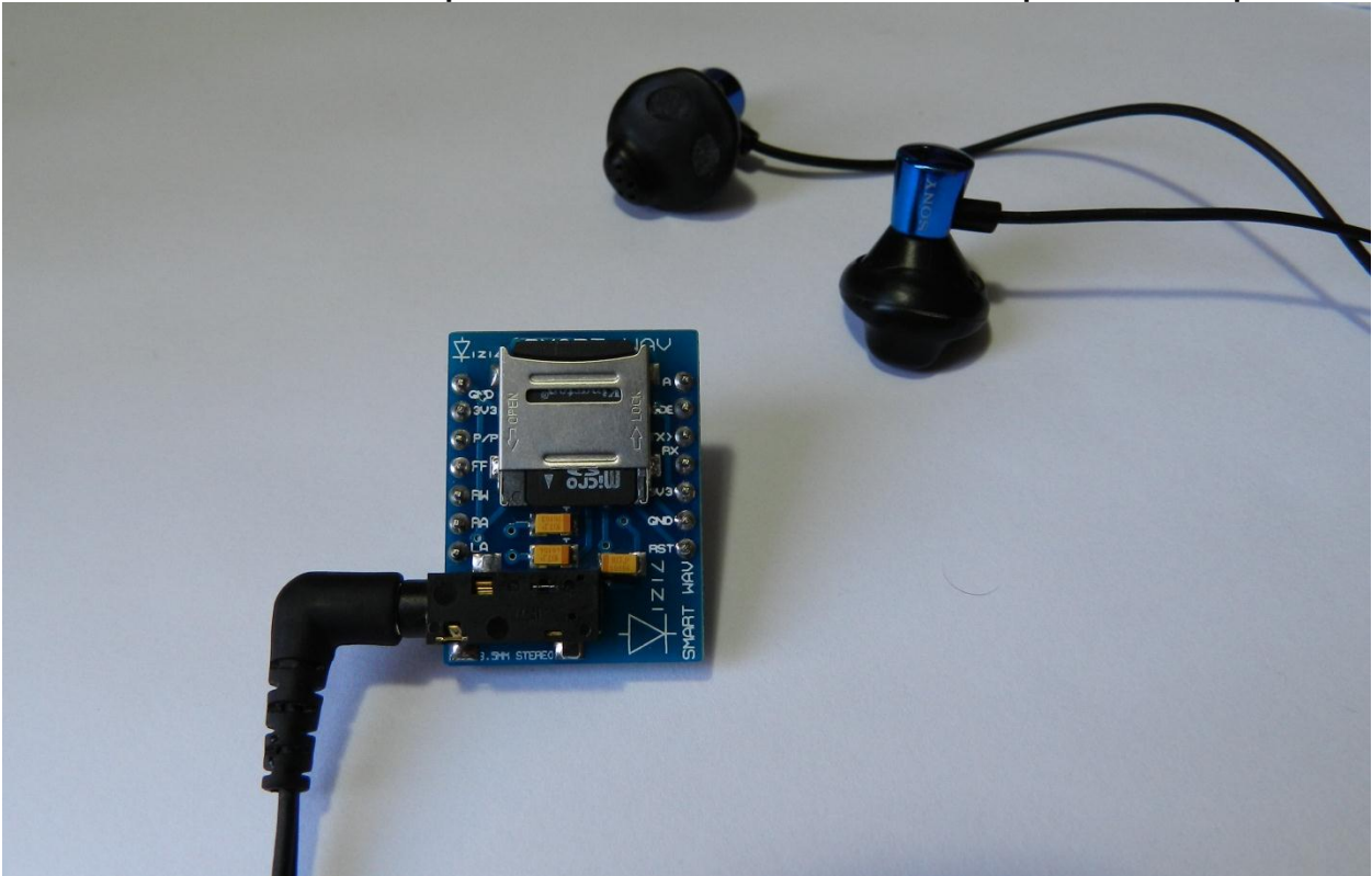
Smart WAV Direct phones connection: Pre-Amplified Outputs
